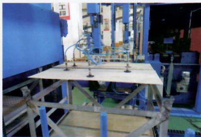
塑料隔板取放 Plastic plate grabbing and placing
